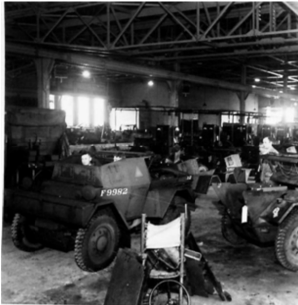
Pictured IWM H_021420 in GB July 1942 A reconditioned Scout Car vehicle number F9982, leaving the Royal Electrical and Mechanical Engineers' (REME) depot for a road test after a complete overhaul
